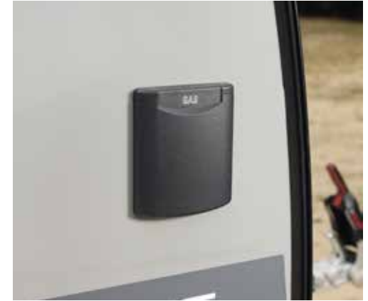
Exterior Gas socket
